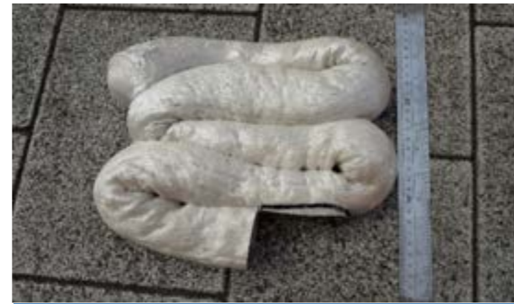
EPS densified using mechanical compression and heat
