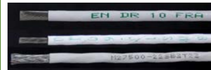
Examples of common aerospace specification wire and cables after laser stripping at the optimised parameters found by analysis.
