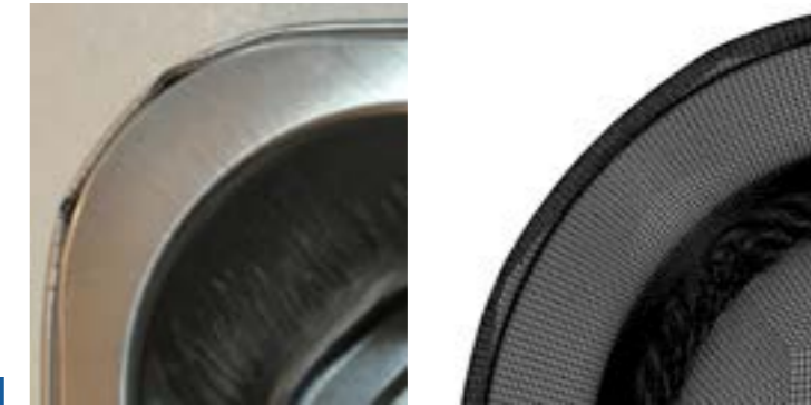
Defects at the corner of (a) the manufactured aluminium food container and (b) the computational model
