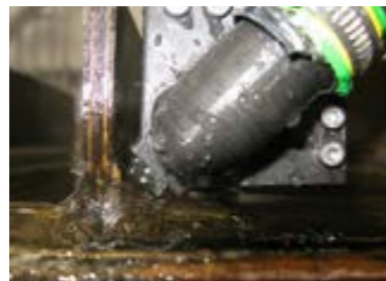
The water jet helps to deliver the signal to and from the surface of the test piece
