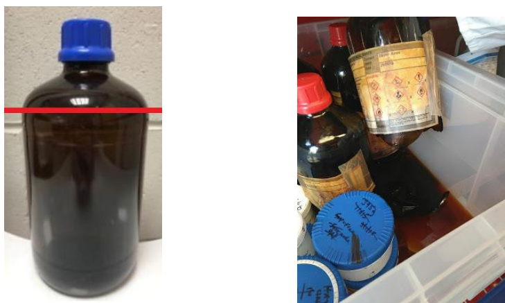
Figure 2. Maximum fill height of a Winchester and the consequences of overfilling and incorrect use.
